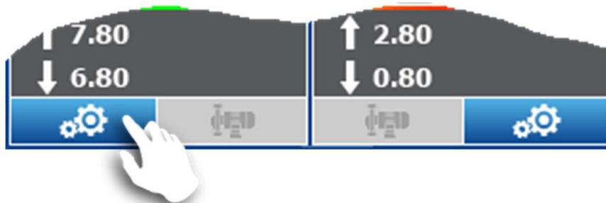
The programming menu of the chosen channel opens (here pH), gives access to the functions of parameter settings of the channel.
